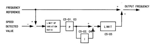
Proportional gain and integral time are approximated in a straight line by motor speed as shown below.
